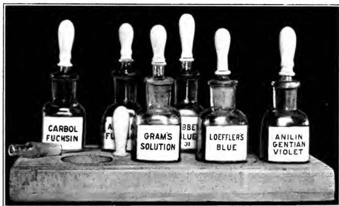
FIG. 137.—Author's staining set. Square bottles are set in square holes in the block. The capacity of each bottle is 30 cc.
